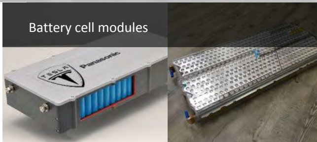
Battery pack (Tesla Model S – 16 modules)
