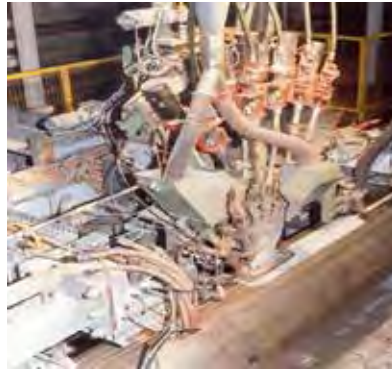
Figure 13. Submerged Arc Welding. (Image courtesy of Tata Steel Tubes)
