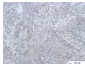
Figure 17. Bainite would be observed at cooling rates between 3 and 20 °C/sec.
