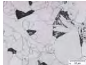
Figure 16. Ferrite and perlite (dark areas) would be observed at cooling rates around 1 °C/sec.
