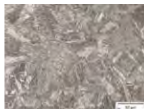
Figure 18. Martensite would be observed at cooling rates exceeding about 30 °C/sec.
